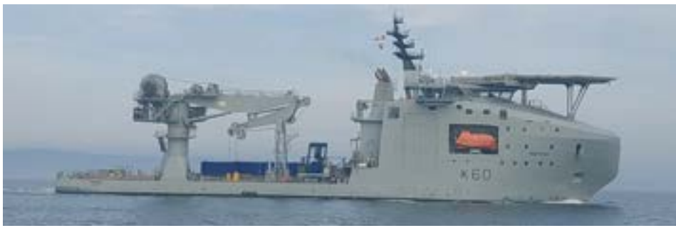
S/M David Meehan took this picture of RFA Proteus sailing from Leith earlier this month. Proteus is a multi-role ocean surveillance vessel of 6,000 tons, and will act as a mother ship for remotely-operated underwater vehicles (ROUVs) and a testbed for new specialist capabilities, monitoring UK waters.
